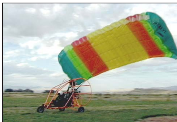
Figure 12-4. A wing lock-out.
