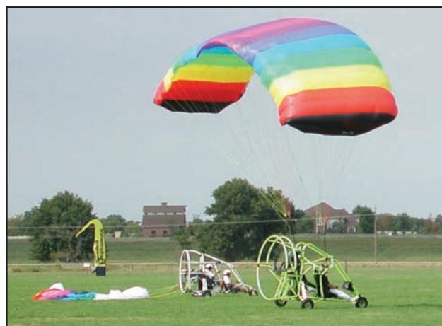
Figure 7-3. Pressurizing, or kiting, the wing.
