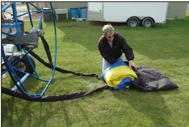
Figure 5-23. With the wing folded, you pull it into the bag.
