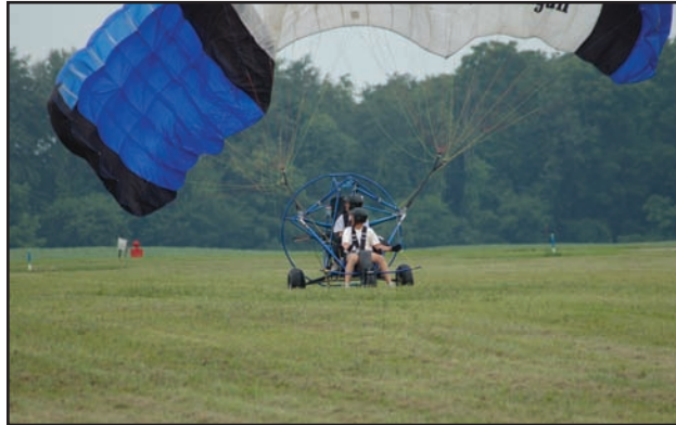
Figure 11-7. Collapsing the parachute.
