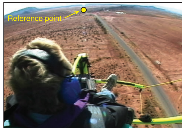
Figure 6-4. Nose reference for straight-and-level flight.
