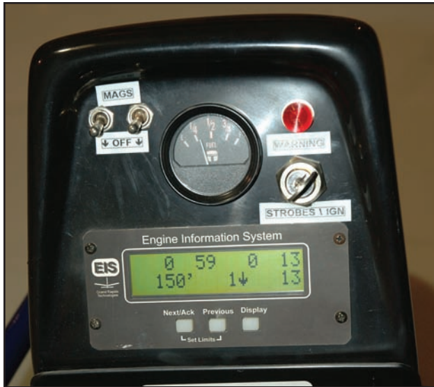
Figure 3-7. Typical engine information system.
