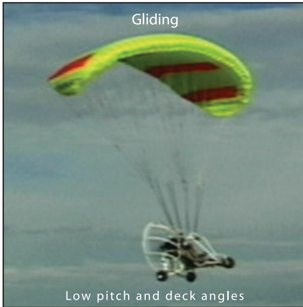
Figure 2-4. Gliding and climbing pitch angles.
