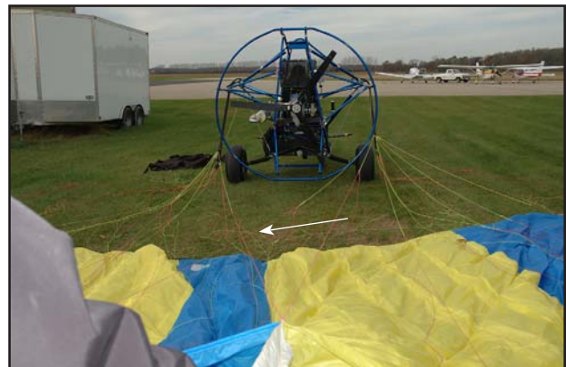
Figure 5-14. “X” in the suspension lines marks the exact center of the uninflated wing.
