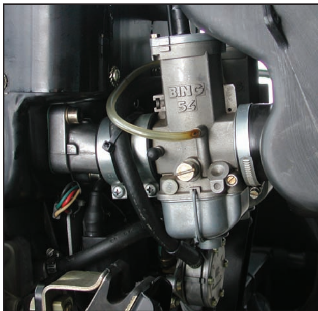
Figure 4-9. Typical 2-stroke carburetor.
