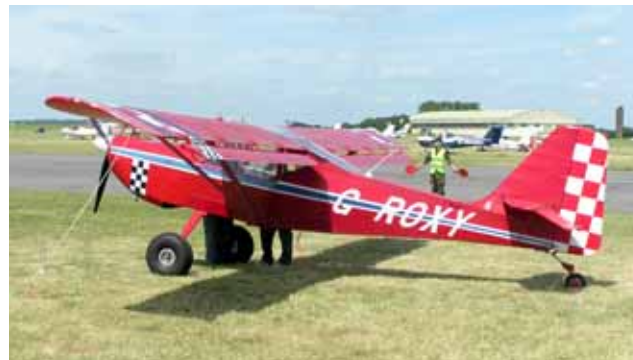
Figure 5-9. Flaperons on a Skystar Kitfox MK 7.
