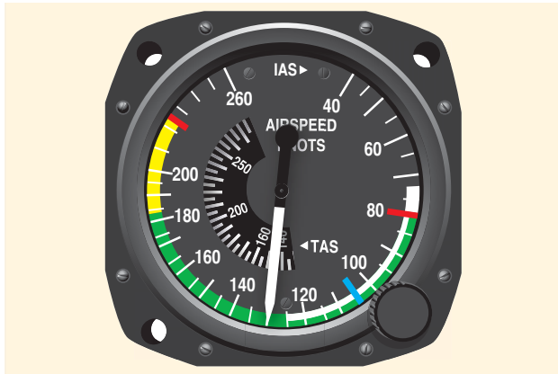
Figure 8-2. Multi-engine airspeed indicator.
