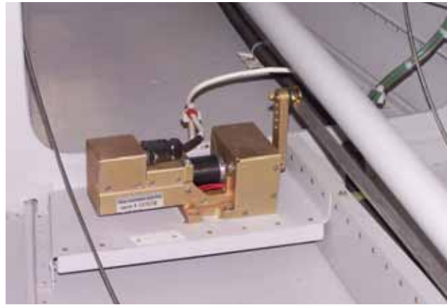
Figure 5-24. Basic autopilot system integrated into the flight control system.
