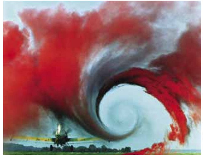
Figure 4-7. Wingtip vortex from a crop duster.
