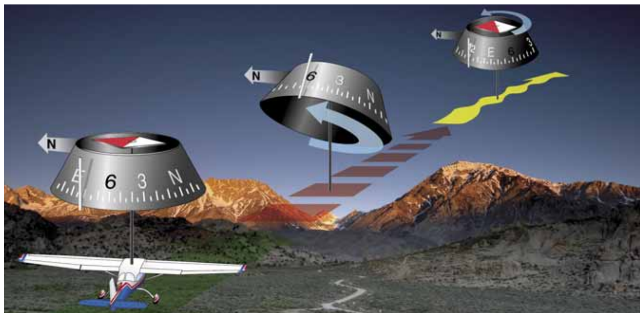
Figure 7-36. Effects of acceleration error.
