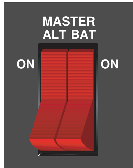
Figure 6-33. On this master switch, the left half is for the alternator and the right half is for the battery.
