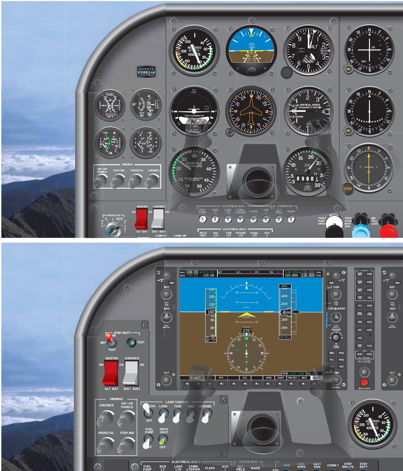
Figure 17-19. Two similar flight decks equipped with the same information two different ways, analog and digital. What are they indicating? Chances are that the analog pilot will review the top display before the bottom display. Conversely, the digitally trained pilot will review the instrument panel on the bottom first.
