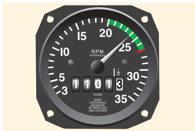
Figure 6-8. Engine rpm is indicated on the tachometer.
