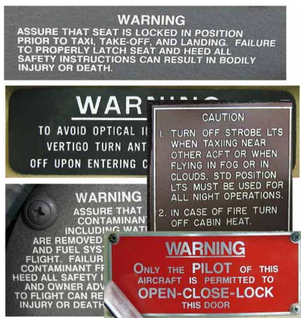
Figure 8-5. Placards are used to depict aircraft limitations.
