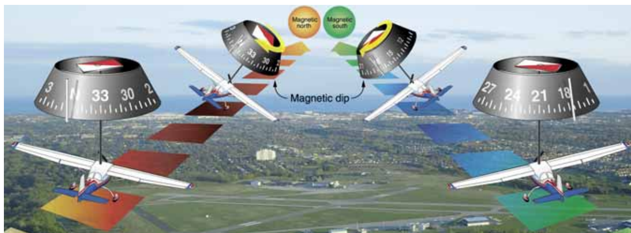
Figure 7-35. Northerly turning error.
