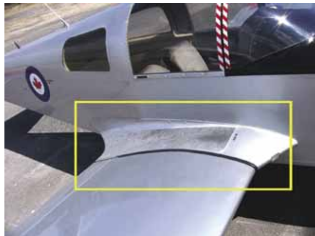
Figure 4-6. A wing root can cause interference drag.
